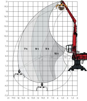
Example lifting capacity range with 10 m straight boom and 8 m stick. Ask for your optimal configuration.
