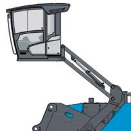
Cab system hydraulically adjustable
